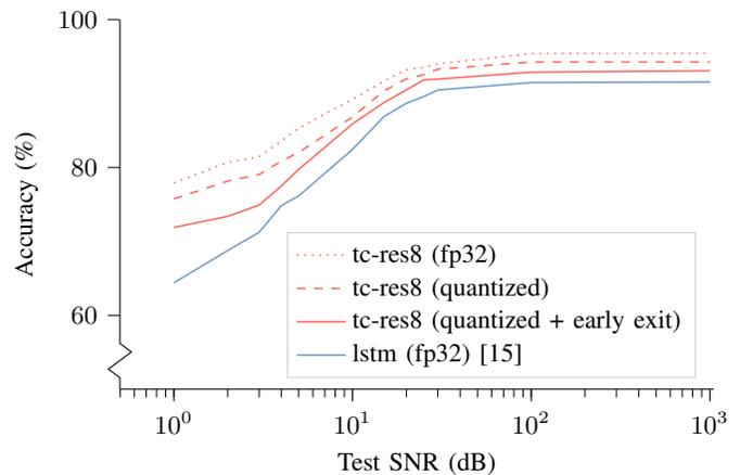
Fig. 14. Behavior in noisy environments compared to the network implemented on a state of the art accelerator [15].
