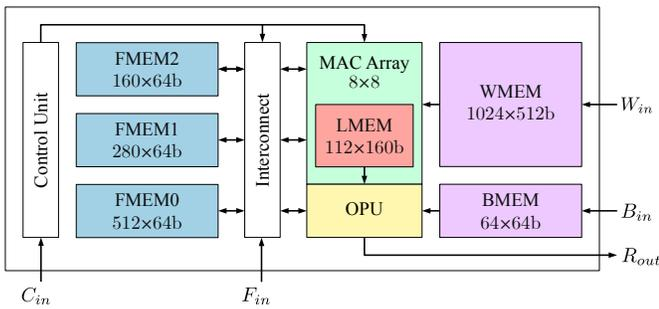
Fig. 5. Overview of the UltraTrail system architecture.
