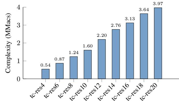
Fig. 10. Computational complexity of different TC-ResNet architectures.
