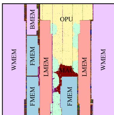
Fig. 15. Die layout of the UltraTrail accelerator in Globalfoundries' 22FDX.
