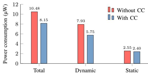
Fig. 17. Impact of conditional computing (CC) on power consumption.
