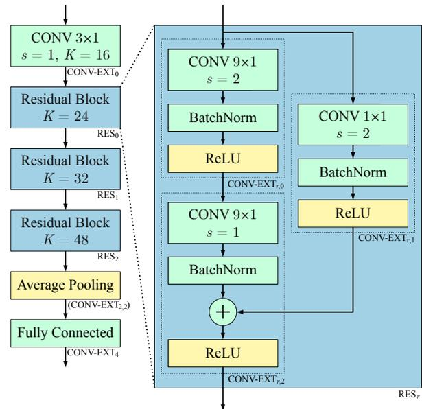
Fig. 1. Example residual network for temporal convolution (tc-res8).
