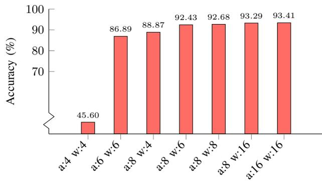
Fig. 11. Effect of varying bit widths for weights ( $w$ ) and activations ( $a$ ) on accuracy.
