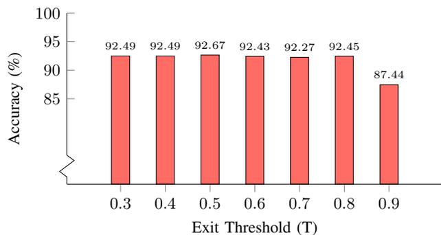
Fig. 12. Accuracy of early exit network tc-res8 with early exits after the first and second residual block under varying thresholds.
