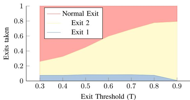
Fig. 13. Distribution of exits taken (exit 1, exit 2, normal exit) depending on a given exit threshold using quantized TC-ResNet8.
