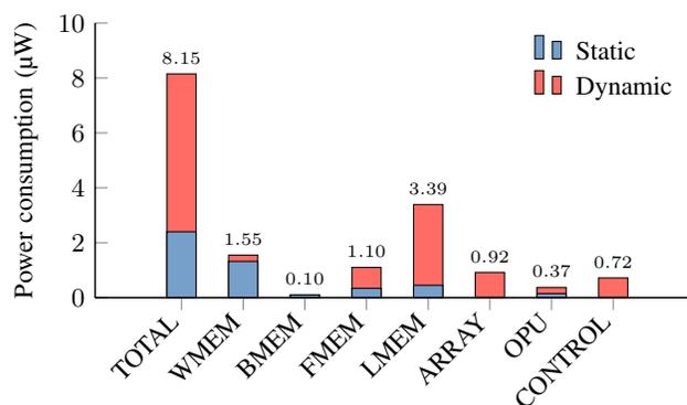
Fig. 16. Power breakdown by components.
