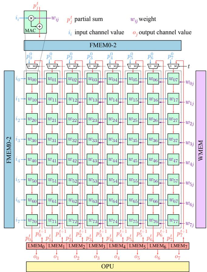
Fig. 6. Schematic view of the MAC array.
