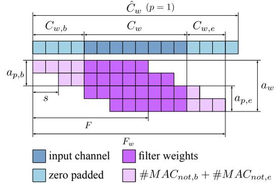
Fig. 8. Depiction of generalized filter applications onto a single input channel.
