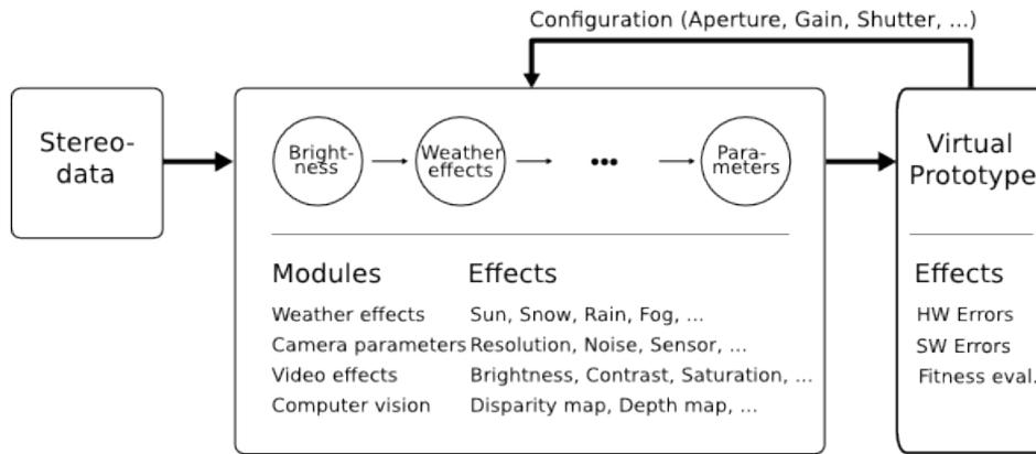
**Figure 1:** Parameters affecting the preparation chain
